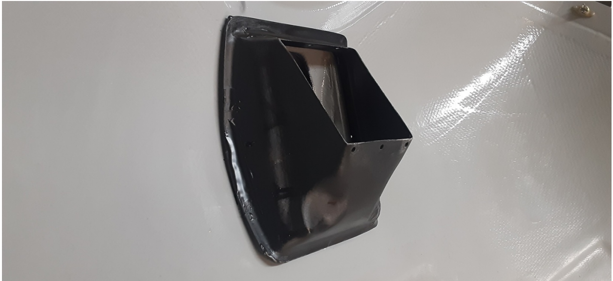
Filter box fabricated and fitted to the inside of cowl. The three holes on the top and bottom of the box are for mounting gap seals which complement the seals shown on the injector box.
